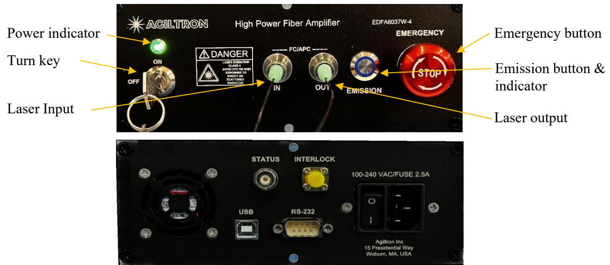
Figure 1: Front and rear panels of EDFA
