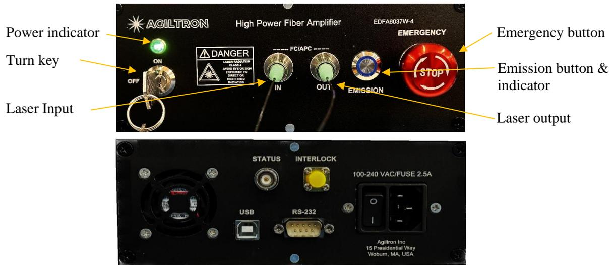
Figure 1: Front and rear panels of EDFA
