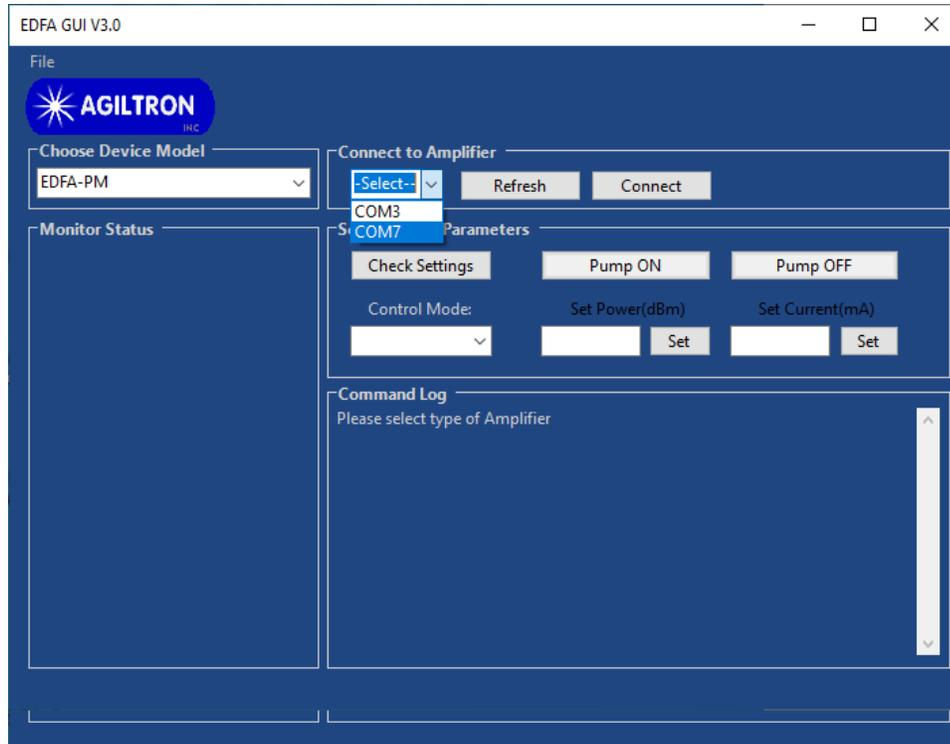
Figure 4: Remote control software: COM port selection.
