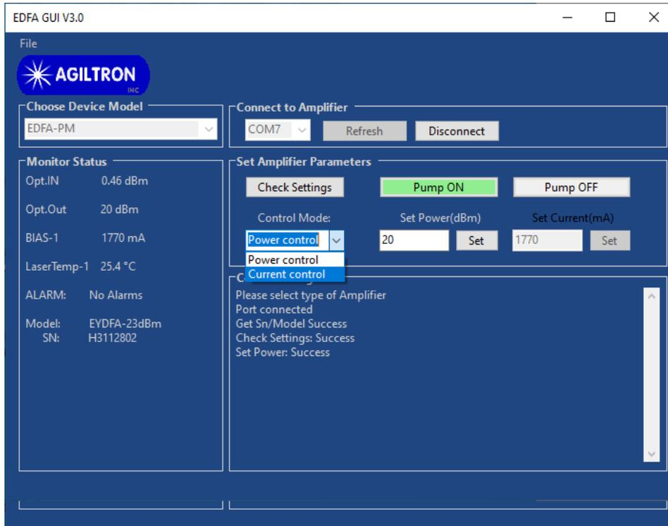
Figure 5: Remote control software: control mode selection
