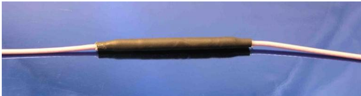
Figure 7. A finished splice (with shrink tube)
